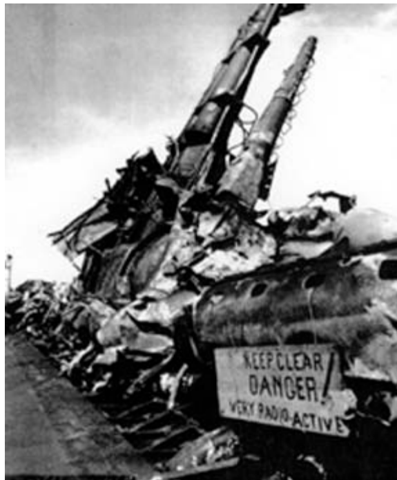
Figure 7. Damage to USS Skate, Able test, operation Crossroads, July 1 st , 1946.
