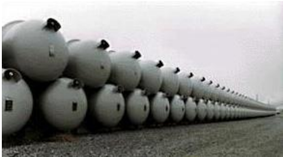
Figure 27. Depleted Uranium (DU) storage cylinders.
