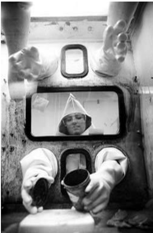
Figure 28. Inert gas plutonium glove box.
