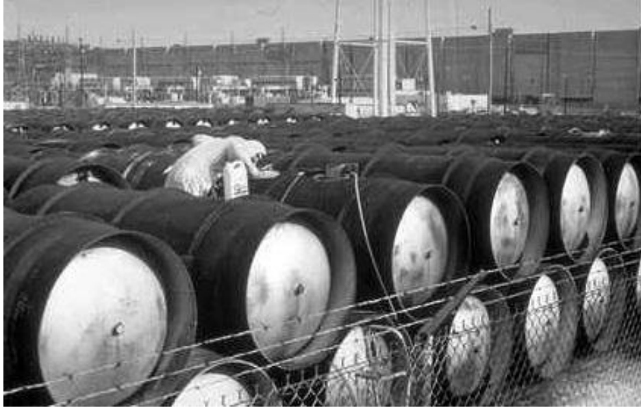
Figure 26. Uranium hexafluoride UF_6 storage cylinders.
