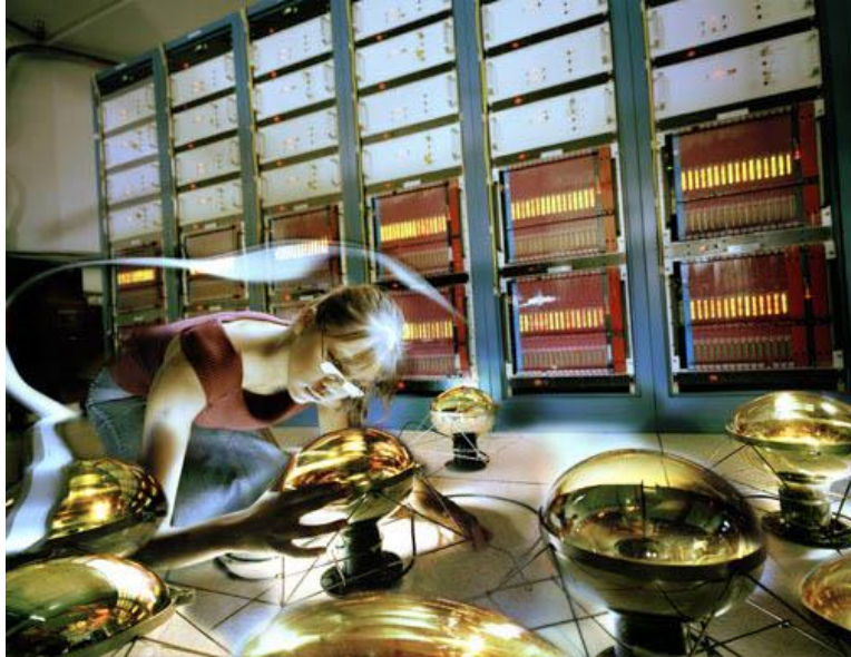
Figure 7. Phototubes being adjusted in the MiniBooNE experiment at Fermi Lab, Batavia, Illinois.
