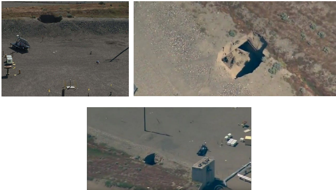
Figure 40. The tunnels were used beginning in the 1950s to store contaminated equipment. The 20 foot wide by 20 foot long cave-in is in an area where the two tunnels join together, possibly as a result of an area earthquake or a quarry blast northwest of the site. A road is being constructed in the foreground.
