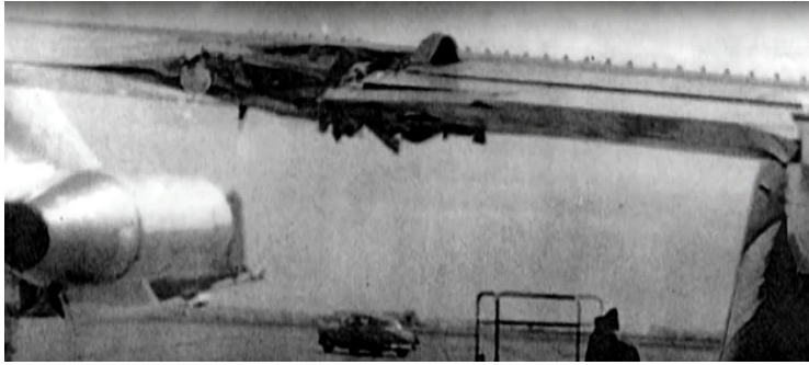
Figure 55. Damaged wing of B-54.
