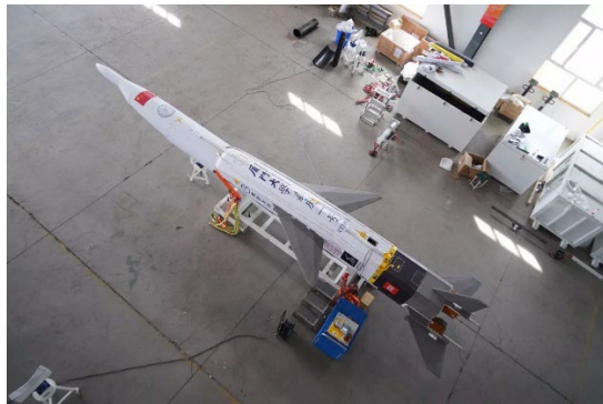
Figure 57. Retrievable “Double Wave Rider” XTER-1 at XIAMEN University flew 400 secs at a height of 27.4 km reaching a speed of Mach 5.5-6.0 which was reduced to Mach 0.35 into a maneuverable glider mode part of the flight. Source: East Pendulum.
