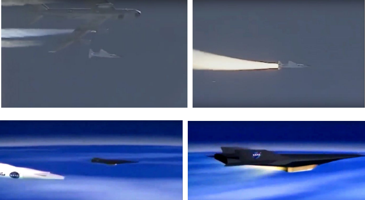
Figure 18. X43-B hypersonic scramjet launch from a B-52 bomber aircraft and solid fuel rocket, Mach 7 speed, March 2004. Carbon/carbon light weight composite material can withstand 3,000 degrees Fahrenheit temperatures. Source: NASA. (Mach 10 = 7,000 mph = 12,000 kph).
