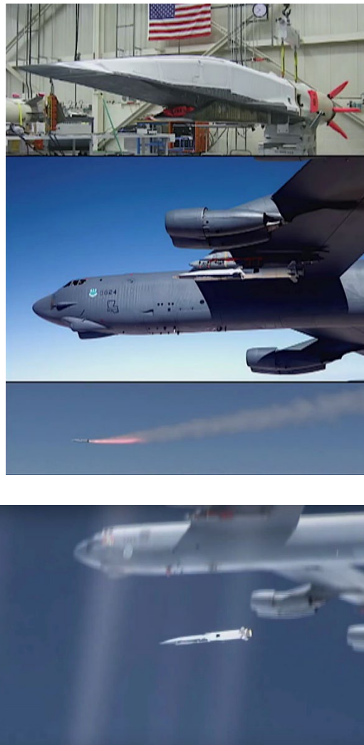
Figure 15. NASA 43A used hydrogen fuel, and reached Mach 6.83 and 9.68 in 2004. Source: NASA.
