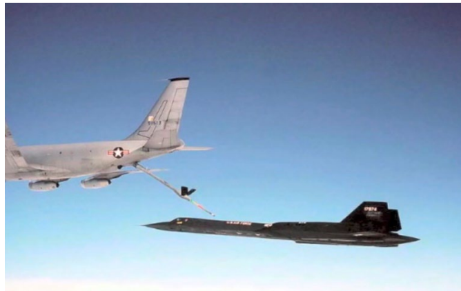
Figure 39. Black Bird, SR 71 spy plane reached Mach 3.6 challenging the “Thermal Barrier” with its titanium instead of Aluminum structure. The SR 71 had to allow for the thermal expansion of its fuel tanks in a preliminary flight allowing for fuel leakage before being refueled ahead of starting its main mission flight.
