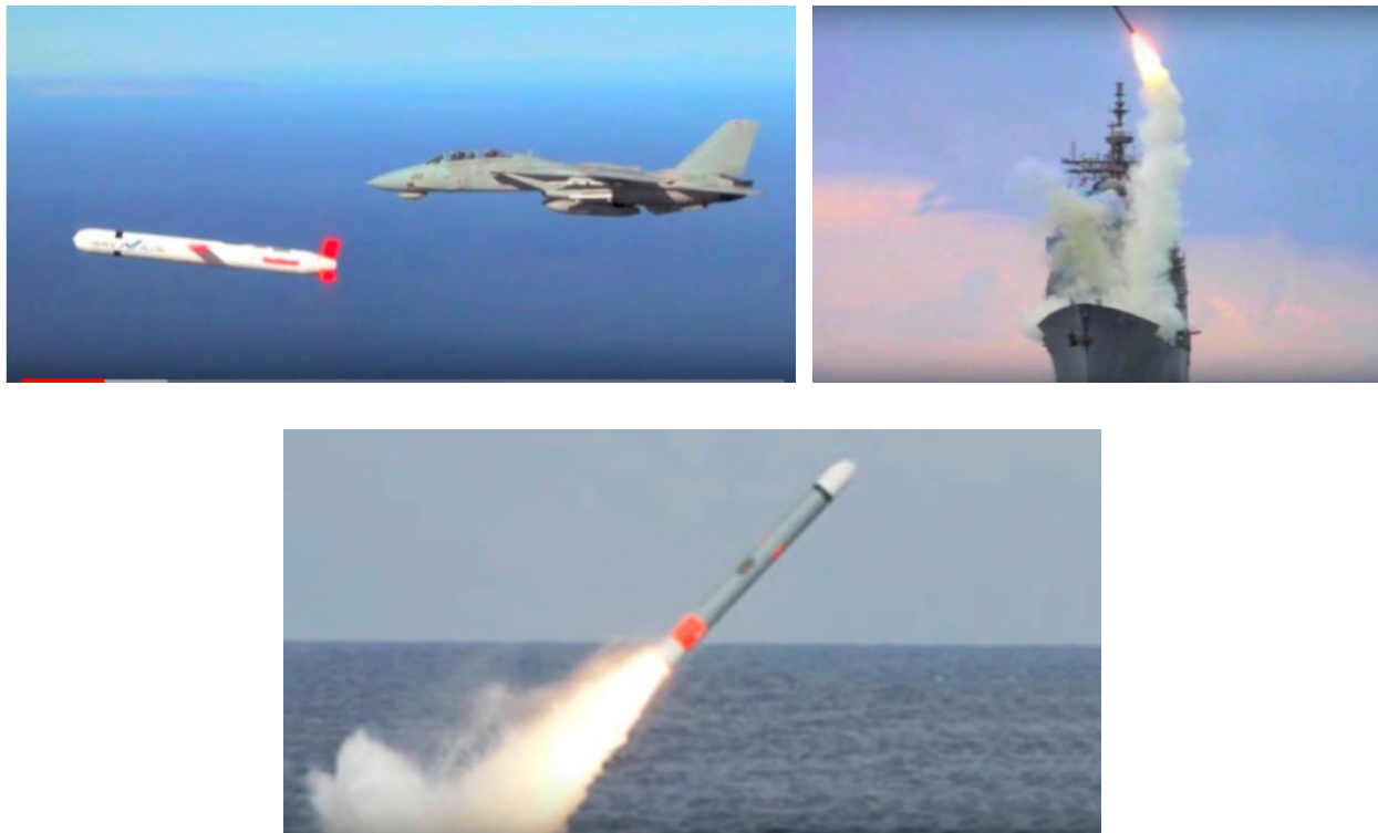
Figure 17. Tomahawk Block IV cruise missile launchable from aircraft, ships or submarines.. It uses sophisticated terrain following and scene-matching electronics plus GPS. The “scenes” are assembled ahead of time and programmed into the computer memory of the Tomahawk. The flight path is predetermined and the scene matching provides the final guidance.
