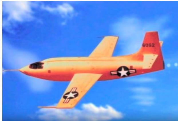
Figure 41. Bell X1 first experimental supersonic, Mach 1 = 1,600 km/hr, manned jet.
