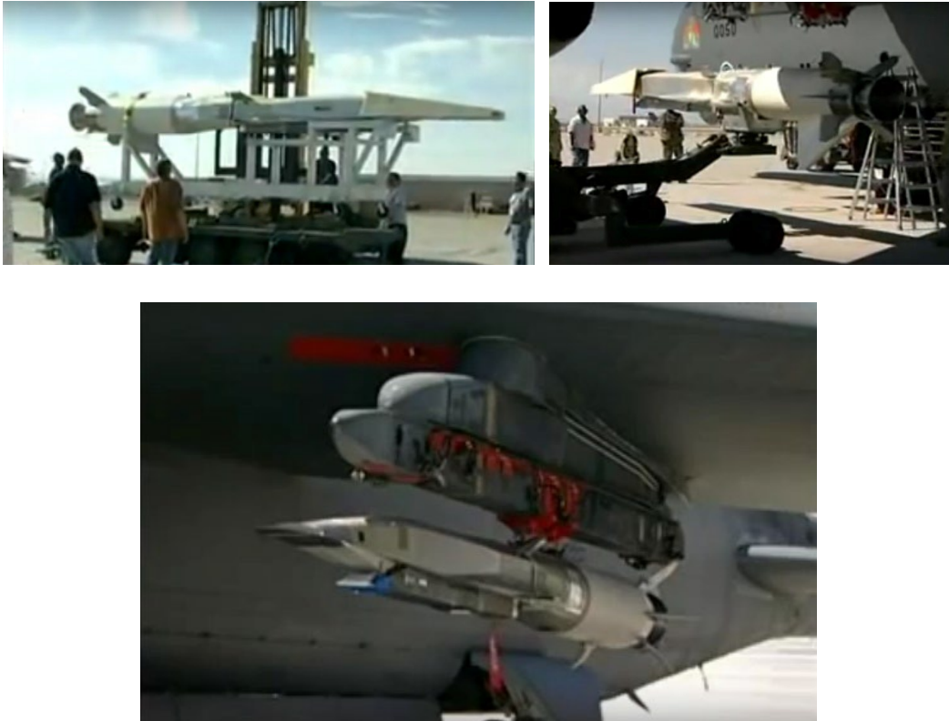
Figure 18. X43-B hypersonic scramjet launch from a B-52 bomber aircraft and solid fuel rocket, Mach 7 speed, March 2004. Carbon/carbon light weight composite material can withstand 3,000 degrees Fahrenheit temperatures. Source: NASA. (Mach 10 = 7,000 mph = 12,000 kph).
