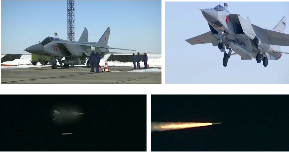
Figure 37. Kinzhal, “Dagger” cruise missile launch from Mig 31BM interceptor has a range of 1,000 kms.
