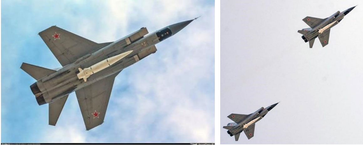
Figure 36. High precision Kinzhal “Dagger,” hypersonic cruise missile launched from the belly of a Mikoyan Mig 31 Foxhound supersonic interceptor jet.
