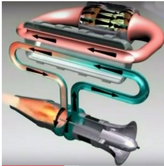
Figure 11. Pratt & Whitney closed cycle nuclear aircraft engine using liquid metal as a heat transfer medium.
