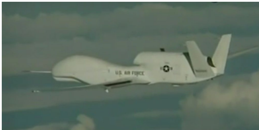
Figure 53. Northrup-Grumman Global Hawk Unmanned Aerial Vehicle UAV a candidate aircraft for nuclear propulsion as it does not need crew shielding. Instrumentation shielding will be required though.
