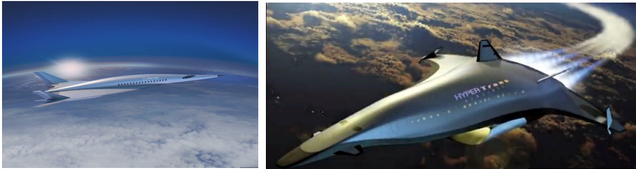
Figure 44. Boeing Mach 5, 95,000-foot hypersonic commercial aircraft concept. The speed of sound drops off with altitude, so Mach 5 at 70,000 or 95,000 feet is a much lower speed than a theoretical Mach 5 at sea level. Source: Boeing.
