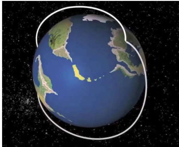
Figure 3. An ICBM South Pole trajectory avoids the installed ABM system.
