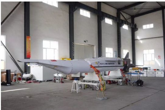
Figure 57. Retrievable “Double Wave Rider” XTER-1 at XIAMEN University flew 400 secs at a height of 27.4 km reaching a speed of Mach 5.5-6.0 which was reduced to Mach 0.35 into a maneuverable glider mode part of the flight. Source: East Pendulum.
