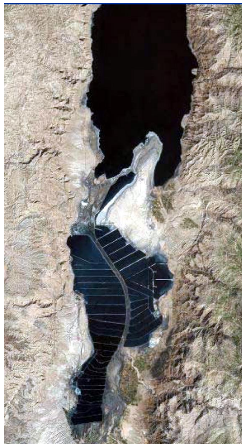
Figure 3. Enhanced satellite picture of the southern edge of the Dead Sea showing the north and south basins and the potash extraction works evaporation ponds in the southern basin. Israel's Dead Sea Works and Jordan's Arab Potash companies mine Dead Sea
