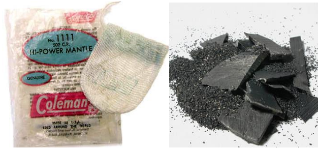
Figure 31. Thorium dioxide with 1 percent cerium oxide impregnated fabric, Welsbach incandescent gas mantles (left) and ThO 2 flakes (right). Yttrium compounds now substitute for Th in mantles.
