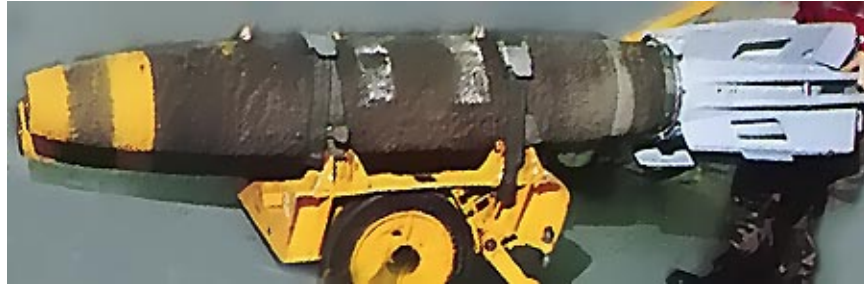
Figure 61. Five hundred pounds Joint Direct Attack Munition (JDAM) on its cart, showing the directional steering and control fins.
