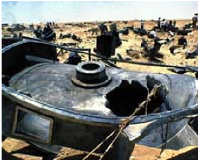
Figure 15. Destroyed vacuum chamber casing of a single experimental Calutron electromagnetic separation device.
