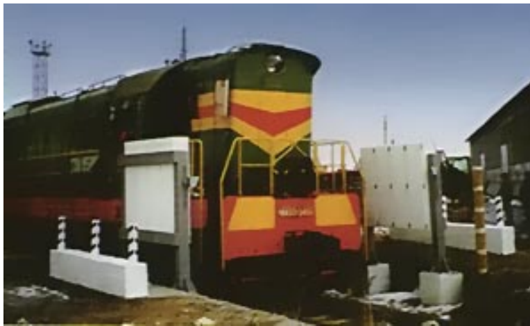
Figure 50. Nuclear materials radiation detector proportional counters portal system for trains.
