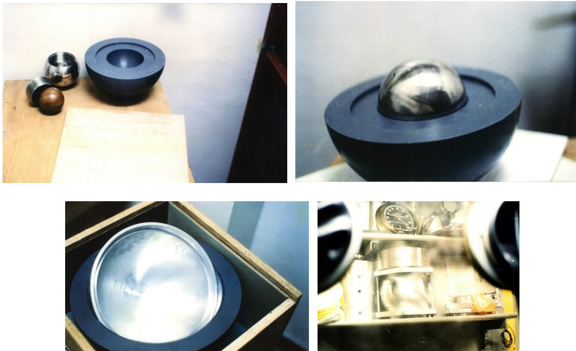
Figure 35. Spherical Pu pit, U tamper/reflector mockup photographs released to Britain's Sunday Times by Mordechai J. C. Vanunu, a dissident whistle-blower advocating a nuclear weapons free world, from Israel's nuclear program. He was a technician who worked at the Israeli Dimona nuclear complex. He revealed some details about Israel's nuclear weapons to the British press in 1986. He was then lured to Italy, kidnapped by Israeli agents, and was confined in the next 18 years in prison in solitary confinement.
