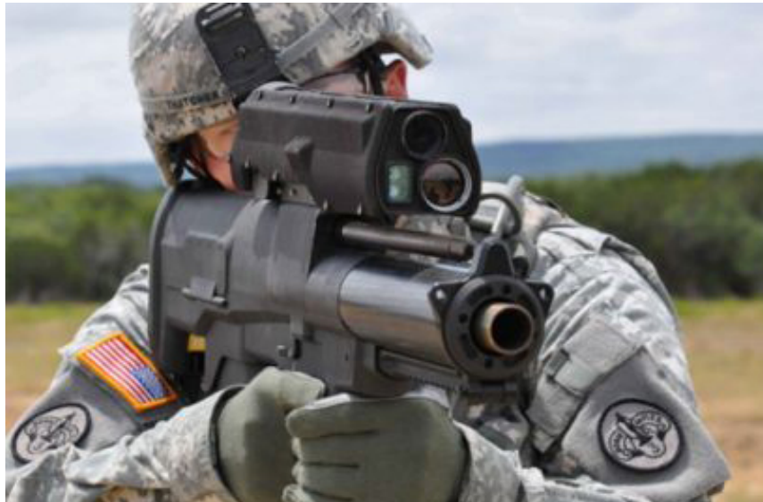
Figure 72. Infantry ATK XM-25 Game-Changer, semi-automatic 25 mm air burst grenade launcher / Individual Airburst Weapon System, IAWS. Photo: DoD.
