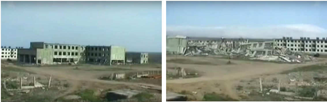
Figure 53. Explosion of Russian thermobaric device. It is characterized by three separate and distinct explosions. The earlier explosion consume the oxygen needed for the subsequent ones and allows the gaseous fuel to expand into the created vacuum before detonating.
