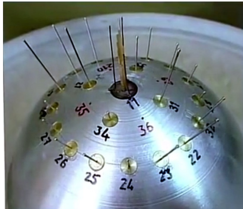
Figure 30. Multipoint initiation implosion experiments on a uranium hemisphere were discontinued in 2003. U^{235} is imploded rather than Pu^{239} , possibly based on Pakistani or North Korean configurations.
