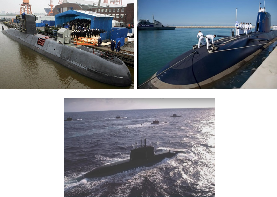
Figure 38. The exclusively-for-export Type 209/1400 class German attack submarine delivered to South Africa, 2005, is not operated by the German Navy (top left). The 3-5 Dolphin class submarines used by the Israeli Navy are based on the Type 209, but are highly modified and enlarged. Flotilla of 5 fuel-cell submarines reportedly armed with nuclear tipped cruise missiles (top right, bottom).
