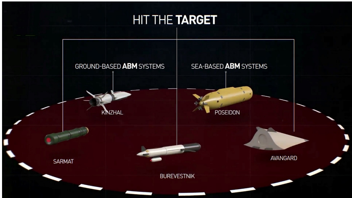
Figure 81. New Russian strategic initiative. The Kinzhal would initially target ground-based ABM systems, and the Poseidon sea-based ABM systems. This opens the way for the Sarmat, Burevestnik (nuclear) and the Avangard to target then undefended targets. The Poseidon is powered by a small reactor and has a top speed estimated at between 60 - 100 knots, with a range of 6,200 miles, and when launched from the Barents Sea or somewhere in the Arctic, can autonomously traverse the North Atlantic, an area where Russia, China, and the USA are staking claims on the natural resources beneath the ocean floor.
