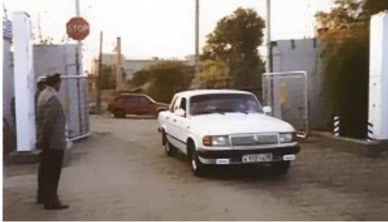
Figure 49. Nuclear materials proportional counter monitors for pedestrians and cars at Astrakhan on the Caspian Sea.
