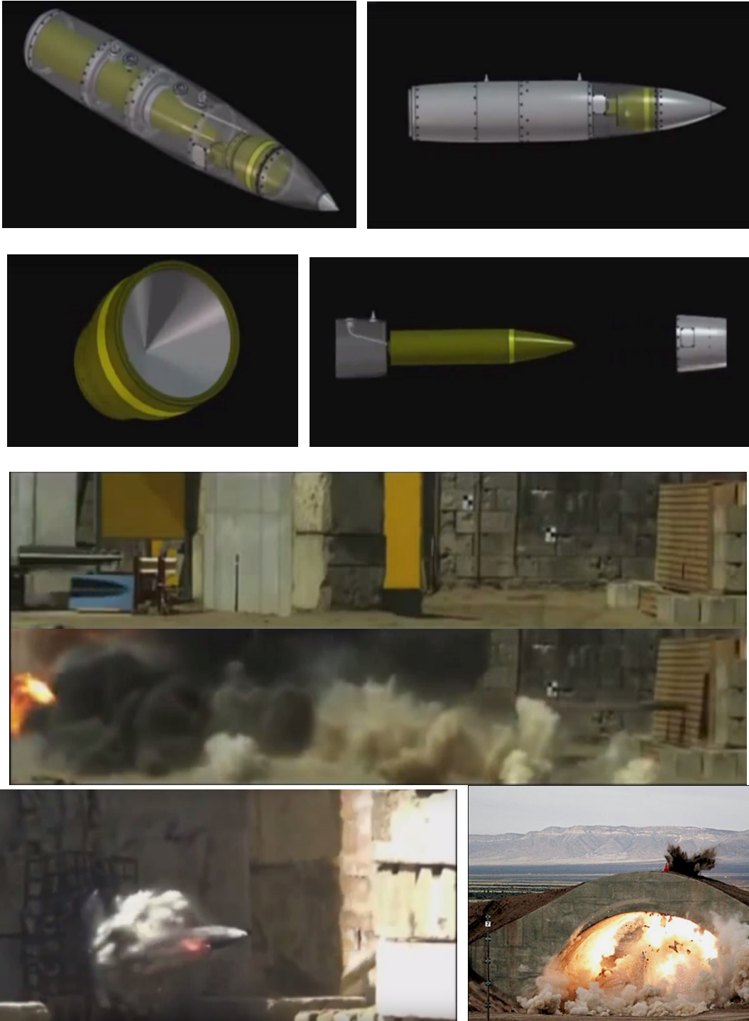
Figure 68. Earth penetrator bunker buster munition consists of a shaped charge front component followed by a hardened case penetrator.
