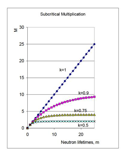
Figure 1. Subcritical multiplication as a function of the neutron lifetimes. k = effective multiplication factor.
