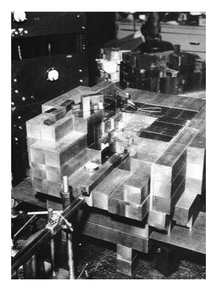
Figure 3. Beryllium blocks used as neutron reflectors for a central core in a subcritical assembly.
