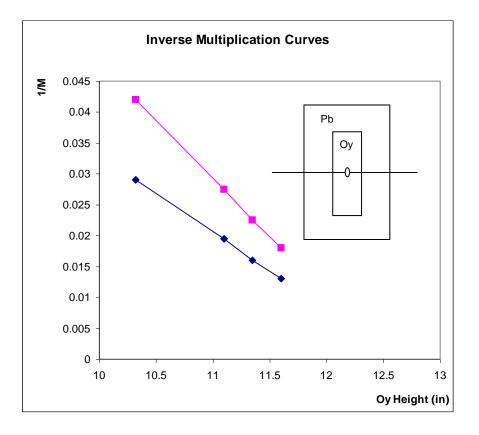
Figure 4. Extrapolation of inverse multiplication (1/M) for 9.9 cm diameter Oralloy cylinder with a 13.3 cm surrounding Pb reflector. Critical height extrapolates to 12.7 inches.
