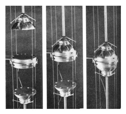
Figure 5. Parts of the Jezebel plutonium critical assembly sliding on wires.
