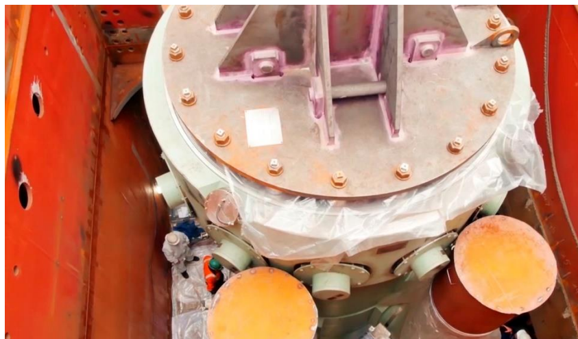
Figure 104. Pressure vessel of icebreaker reactor.
