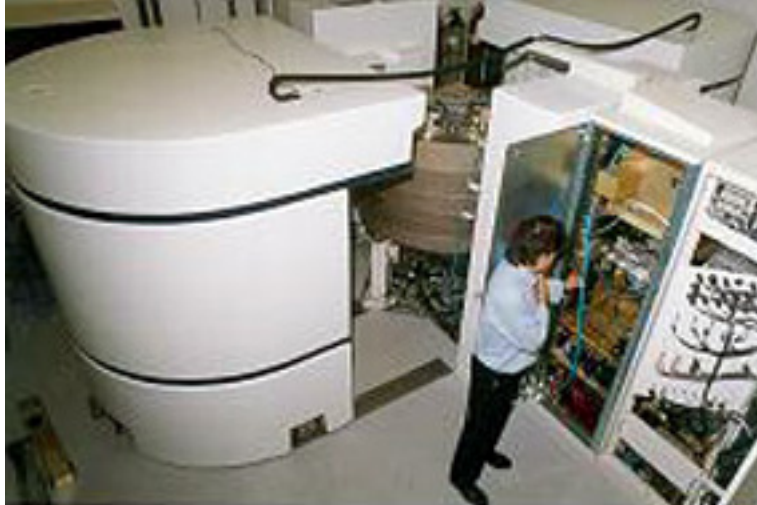
Figure 2. Cyclotron for the production of the isotopes used in PET scanning.
