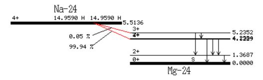
Figure 73. Decay diagram of Na<sup>24</sup>.
