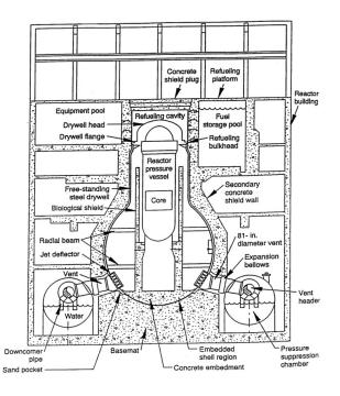
Figure 40. Primary and secondary containments configuration at Fukushima plants.
