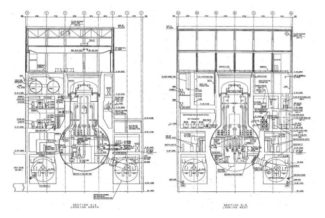
Figure 44. BWR Mark I, light bulb design showing the toroidal steel pressure suppression pool, and the gate between fuel storage pool and reactor top. Source: GE, Japan Ministry of Economy, Trade and Industry, METI, Tepco.
