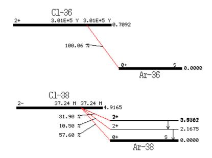
Figure 74. Decay diagrams of the Cl<sup>36</sup> and Cl<sup>38</sup> isotopes.
