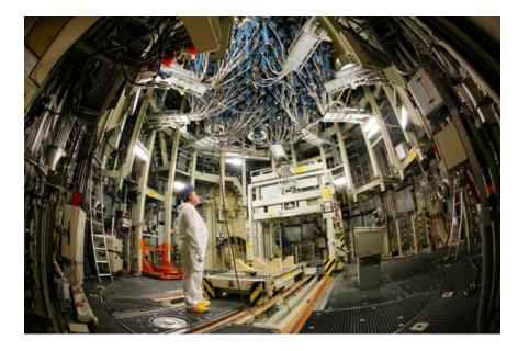
Figure 92. Control rod drives at the bottom of the Krümmel BWR reactor near Hamburg, Germany that went into operation in 1984.
