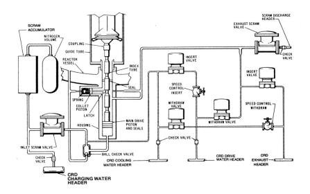
Figure 65. BWR control rod drive mechanism at the bottom of a BWR reactor vessel showing the control rod graphite seals location [2].
