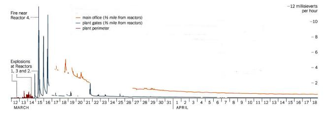
Figure 69. Effective dose rate measurements at main office, plant gates and plant perimeter. Source: Tepco, NY Times.
