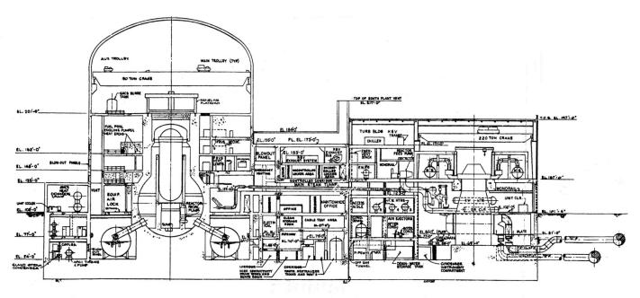
Figure 45. Cutout through containment and turbine hall showing the location of the fuel storage pool in a typical BWR. Plant systems below grade level and hence affected by flooding from the tsunami event include pumps and electrical components. The dry well includes a sump. Any leaking corium material through the control rod seals could interact with the sump water as well as the concrete mat causing a steam explosion, then becoming embedded in the concrete. Source: GE.
