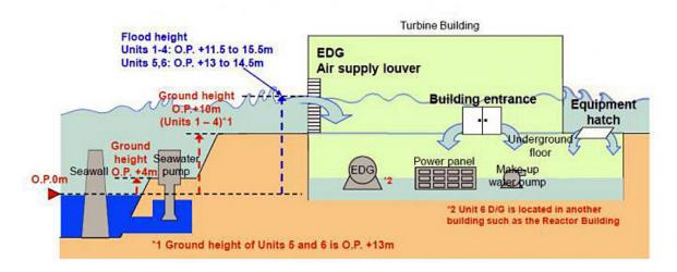
Figure 9. Inundation paths of major buildings at Fukushima plants. EDG: Emergency Diesel Generator. Source: Tepco.
