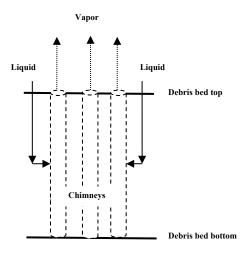
Figure 76. Debris bed chimneys cooling.
