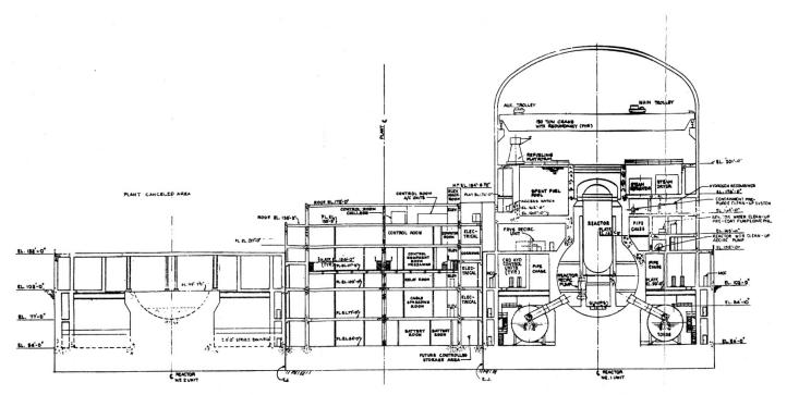
Figure 46. Perpendicular cutout through the containment structure showing the location of the storage batteries. The gate and other connections between the fuel storage pool and the top of the core may have sustained damage as a result of the earthquake and caused leakage of the pools' cooling water. Source: GE.
