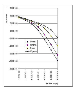
Figure 38. Decay heat power release for a 3,000 MWth Light Water Reactor, LWR for different operational times. The decay heat generation power decreases rapidly within a few days after shutdown.
