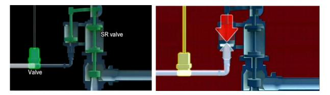
Figure 20. Battery-operated auxiliary valve releases nitrogen pressure to open safety relief valve to vent the containment of hydrogen and steam failed to operate because of unexpected high pressure in the containment that countered the nitrogen pressure. Operators tried to use connected car batteries to operate it unsuccessfully.
