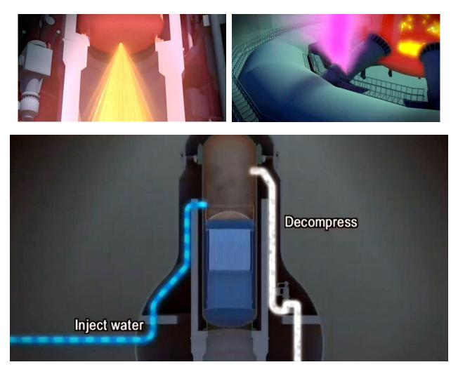
Figure 41. Depressurization of reactor vessel to allow Low Pressure Coolant Injection (LPCI) System to inject water at a high rate into reactor vessel..
