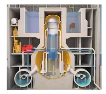
Figure 54. Units 2 and 3 had decay-heat cooling provided by steam-driven turbo-pumps rejecting the decay heat into the pressure suppression pool. They operated for 24 hours until batteries providing power to the control valves were depleted or flooded. Both units underwent hydrogen explosions. Source: Institut de Radioprotection et de Sûreté Nucléaire (IRSN).
