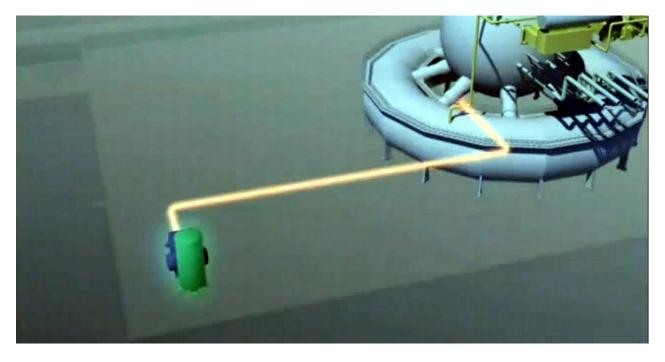
Figure 23. Compressed air containment venting valve failed to operate because of suspected loss of pressure in compressed air lines due to earthquake damage.
