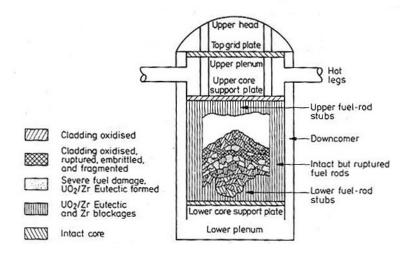
Figure 75. Debris bed resulting from the core damage in the Three Miles Island accident.
