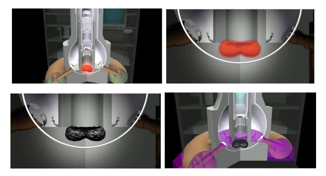
Figure 43. Molten corium material leaked through the control rods graphite seals into the dry well in the primary containment vessel. Dry well flooded through water injection from the top of the core. Source: Tepco.
