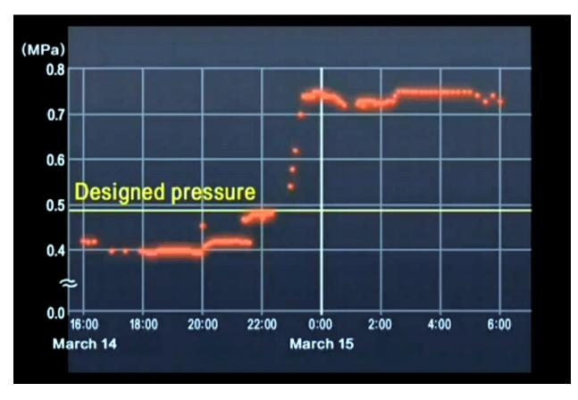
Figure 18. Increase in drywell pressure.
