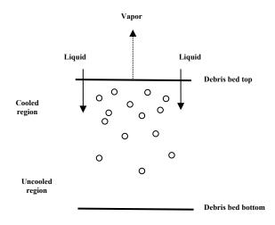
Figure 77. Closed bed debris bed cooling.
