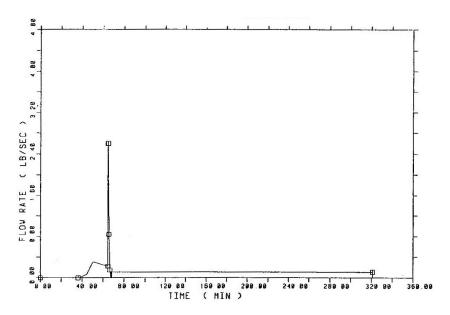
Figure 63. Hydrogen release rate was correlated with a pressure pulse inside the containment structure in the Three-Mile Island Accident. The hydrogen pulse did no discernible damage to the containment structure.
