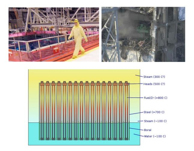
Figure 50. Spent fuel storage pools (top) showing fuel assembly being moved through gate between pool and reactor top. Steam emanating from fuel storage pool in unit 4 on March 15, 2011, under the loading crane showing at the center of the picture.
