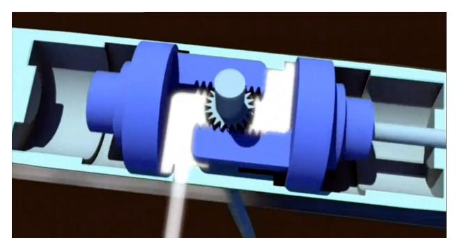
Figure 22. Remote controlled compressed air safety relief valve. Failed to operate due to pressue loss in the compressed air lines.
