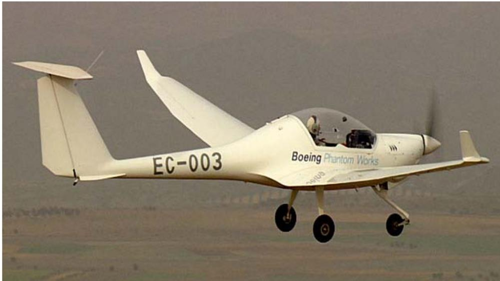
Figure 1. Hydrogen Fuel cell Aircraft designed by the Boeing Company Research And Technology (BRAT) division; formerly Phantom Works was first flown in Spain.
