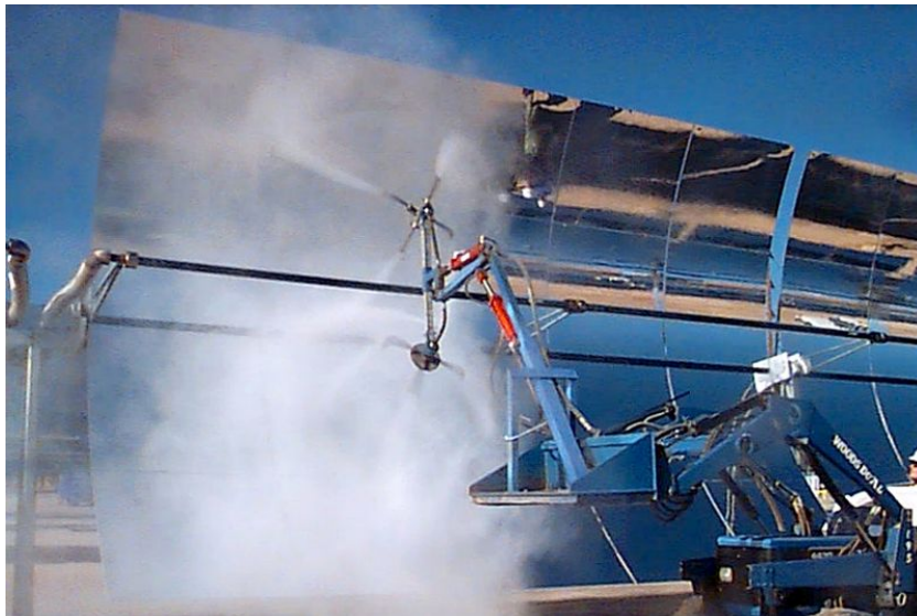
Figure 4. Parabolic trough mirrors washing process.
