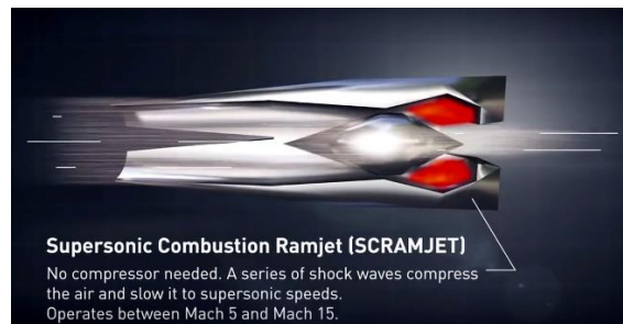
Figure 98. Operation of a ramjet/scramjet engine.
