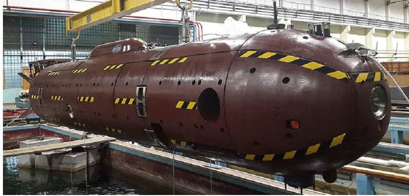
Figure 101. Autonomous Klavesin 2R PM nuclear-powered drone under construction. Submarines are usually designed to be as quiet as possible. The Status-6 would not need to be silent, due to its speed that cannot be matched by existing torpedoes, and since it is unmanned, the Unmanned Underwater Vehicle (UUV) is capable of diving to depths no other submarines can.
