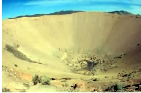
Figure 67. The Sedan underground 105 kT TNT equivalent cratering explosion, July 6, 1962. The release of Cesium 135 and Argon 37 are indicative of underground nuclear explosions.
