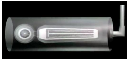
Figure 33. Castle Bravo device used the Ulam-Teller configuration with a uranium tamper generating 80percent of the yield.
