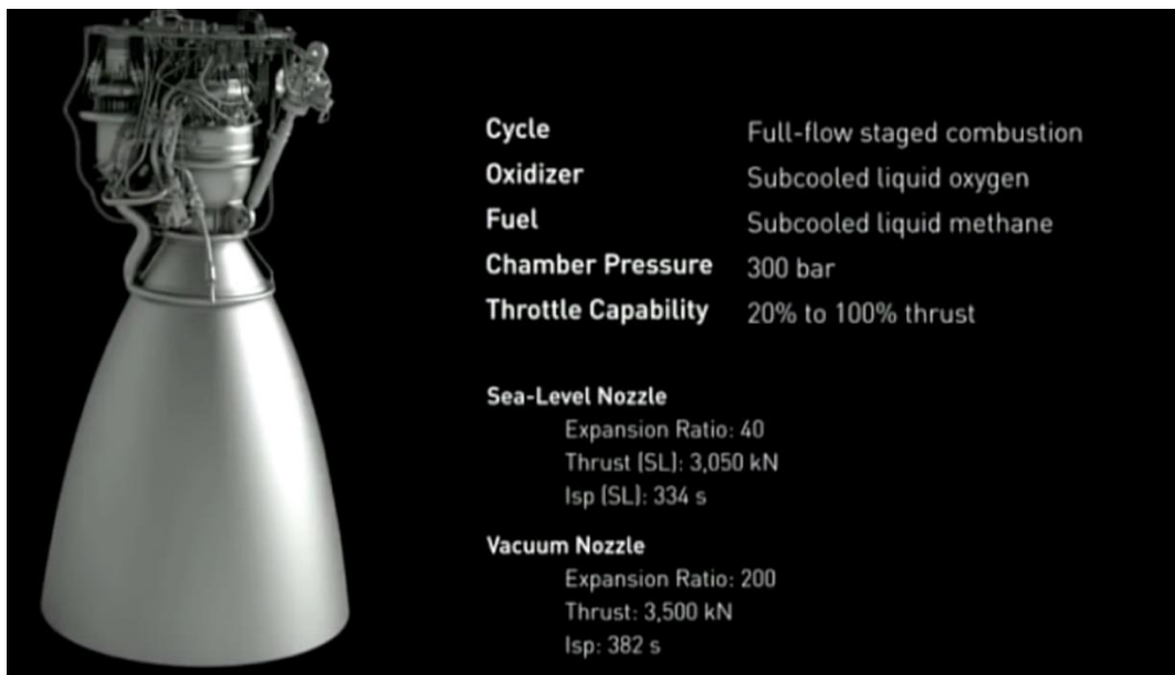
Figure 43. Raptor engine design. Specific impulse of 334-382 is predicted. Source: Space X.
