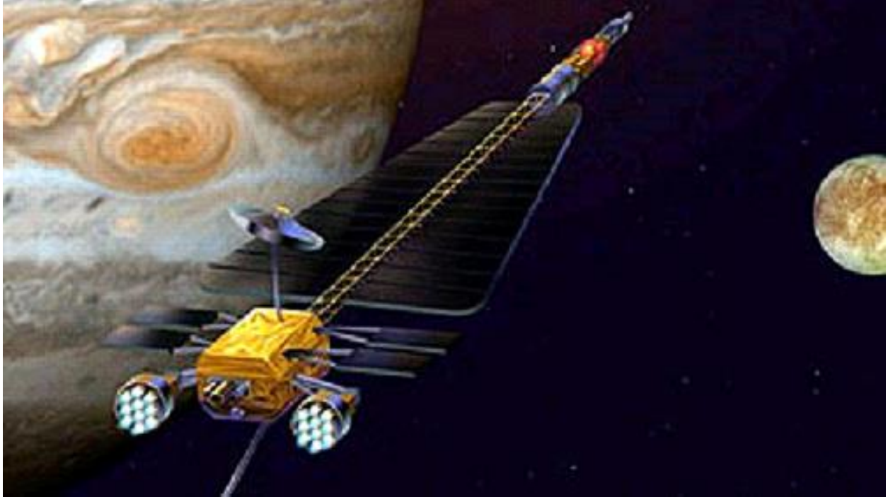
Figure 15. Prometheus ion thruster conceptual design. Source: NASA.
