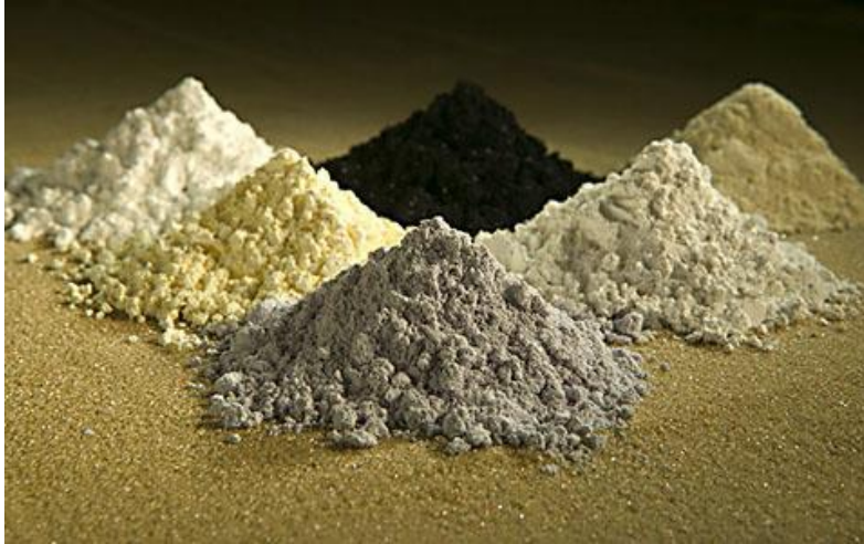
Figure 4. From top center, oxides of praseodymium, cerium, lanthanum, neodymium, samarium and gadolinium. Source: USDA.
