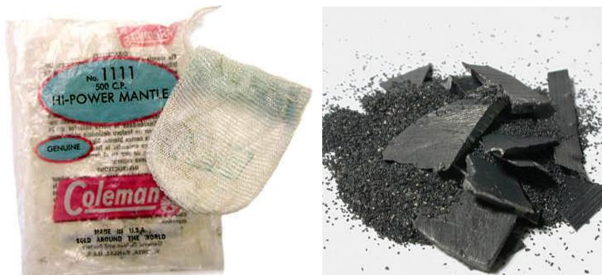
Figure 5. Thorium dioxide with 1 percent cerium oxide impregnated fabric, Welsbach incandescent gas mantles (left) and ThO 2 flakes (right). Yttrium compounds now substitute for Th in mantles.
