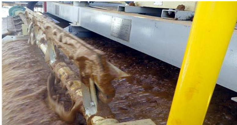
Figure 32. Flotation cells with initial feed.
