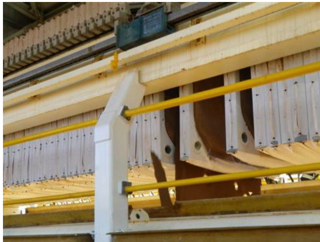
Figure 34. Concentrate cake discharging from filter press.
